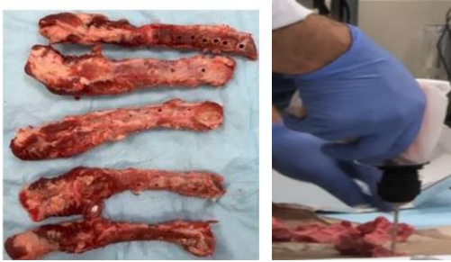
Fig. 2 Setup of experiment. (Left) Five porcine rib bones with 4 samples collected from each bone. The first 2 consecutive samples were obtained using the MR compatible bone biopsy pneumatic drill. The next 2 consecutive samples were obtained using the standard battery powered bone biopsy drill.
