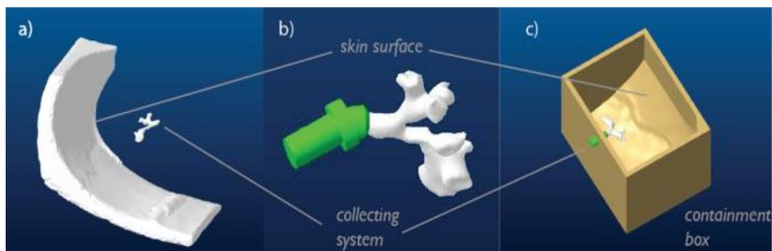
**FIG. 1.** (a) Reconstructed left kidney collecting system image with overlying skin surface from a CT scan using 3DSlicer, (b) CAD model of shaft connected to the collecting system that preserves the original orientation relative to the skin surface, (c) CAD model of the containment box with the skin surface as its base.
