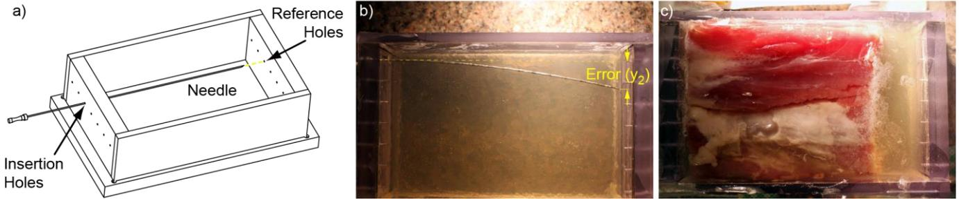
Figure 2: The setup: a) experiment box and b) targeting error measurement example, c) box with ex-vivo tissues fixed in gelatin (deepest side clear for measurements).
