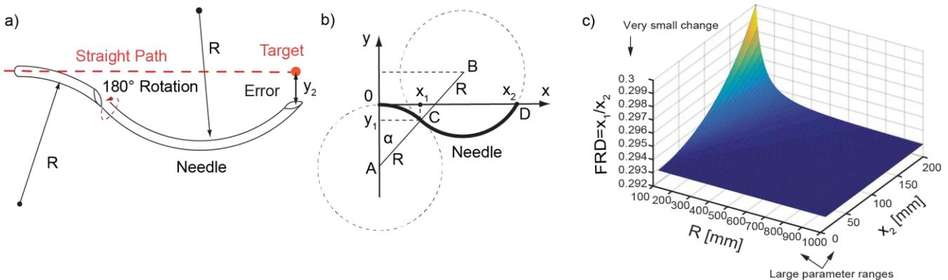
Figure 1: a) Bevel point needle inserted to a depth, rotated  $180^\circ$ , and inserted further, b) Needle path that returns the needle point on the straight trajectory at the depth of the target, c) The needle flip depth ratio (FDR) exhibits very little variation (0.293 - 0.300) for a wide range of its two parameters  $x_2$  and  $R$
