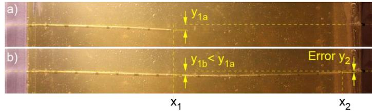
Figure 3: Two photos of an 18Ga needle inserted in gelatin:
