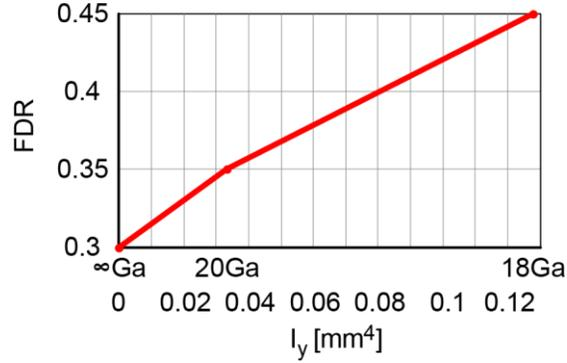
Figure 4: FDR coefficient as a function of the needle cross section moment of inertia,
