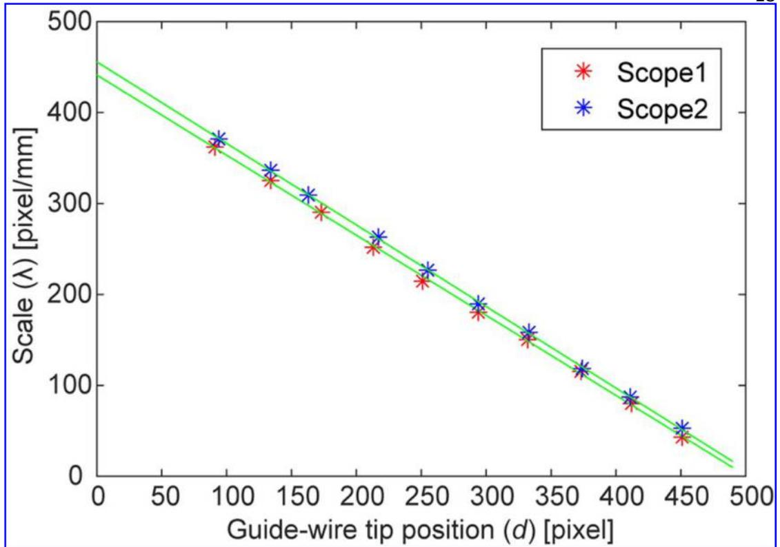
Figure 2. Calibration results of two ureteroscopes. Red and blue asterisks indicate measurement values of the scopes. Green lines indicate linear regression results.
