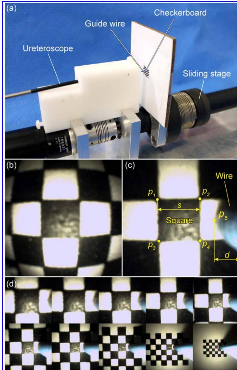
Supplemental Figure 2. Ureteroscope calibration; (a) experimental setup, (b) original ureteroscopic image (distorted), (c) processed image (undistorted), and (d) checkerboard images captured at different positions. The checkerboard was translated to 10 locations ( $D_i, i = 1 - 10$ ), and its images were captured at each position, as shown in Figure 2(d).
