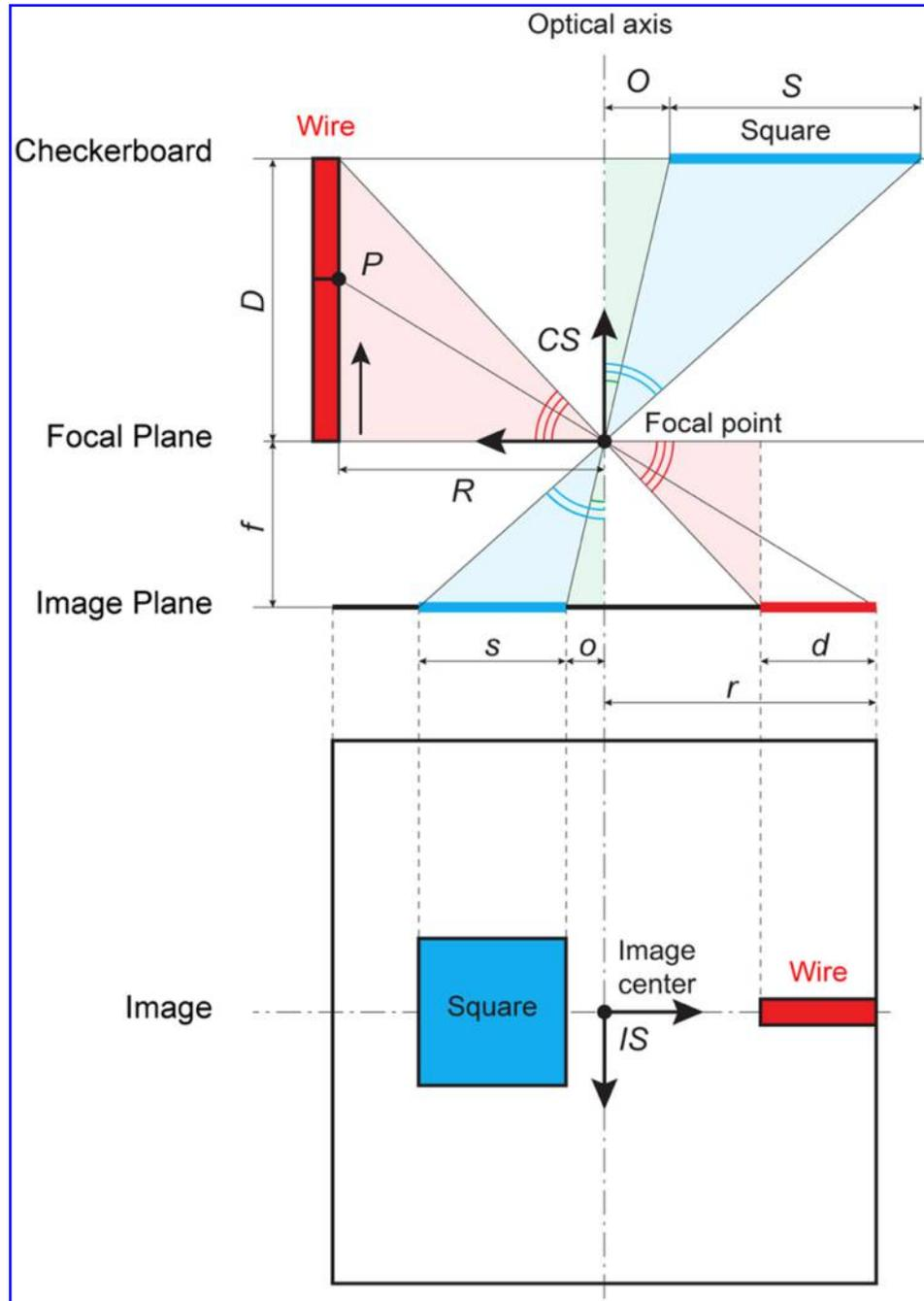
Supplemental Figure 1. Displays a schematic of measurement principle. The physical space (camera space, CS) at the top side and the image space (IS) at the bottom. A square of the board having the size  $S$  [mm] and the horizontal offset of  $O$  [mm] is shown, at a distance  $D$  [mm] from the focal plane. The  $s$  are variables and other are constant parameters.
