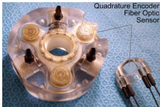
Fig. 1. PneuStep motor used in the robot.
