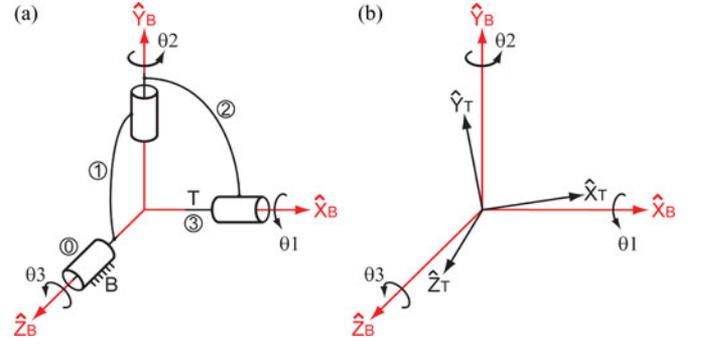
Fig. 2. (a) Symbolic representation of the RCM3 mechanism implementing Z-Y-X Euler angles and (b) Fixed frame X-Y-Z rotations of its tool frame {T} in the fixed base frame {B}.
