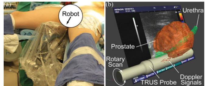
Fig. 10. (a) 4-DoF robot at the beginning of prostatectomy, before docking the daVinci robot and (b) postoperative 3-D reconstruction of pelvic structures based on intraoperative ultrasound scans.
