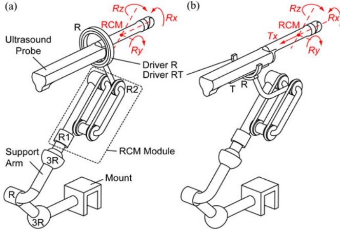
Fig. 1. Kinematic diagram of the robots: (a) 3 DoF with R driver and (b) 4 DoF with RT driver.
