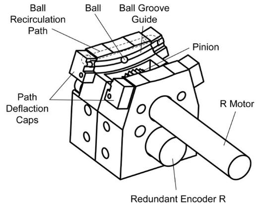
Fig. 6. Ball circulation path within the rotary guide.
