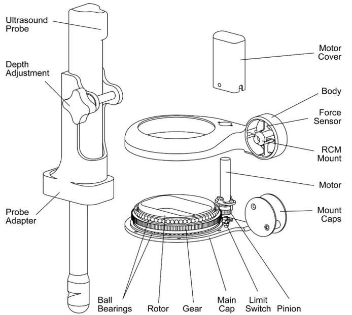
Fig. 4. Ultrasound driver R: exploded view.
