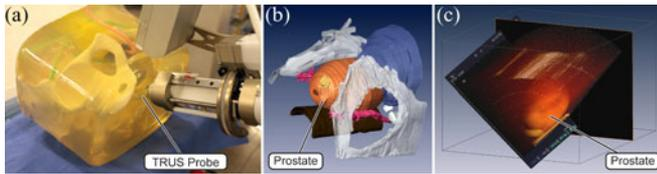
Fig. 8. (a) Pelvic mockup with a TRUS probe supported by the 4-DoF robot, (b) postprocessed 3-D reconstruction from ultrasound images, and (c) 3-D representation of the prostate using volume rendering.
