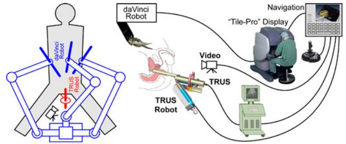
Fig. 9. Schematic setup for T-RALP.
