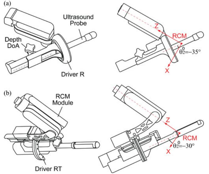
Fig. 3. Ultrasound robots with (a) 3 DoF and (b) 4 DoF.
