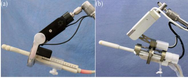
Fig. 7. (a) 3-DoF and (b) 4-DoF ultrasound robots.
