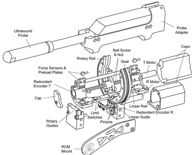
Fig. 5. Ultrasound driver RT: exploded view.
