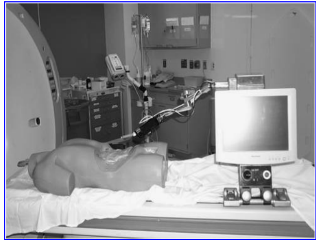
FIG. 2. Computer-assisted navigation device with the infrared tracking device in the background.
