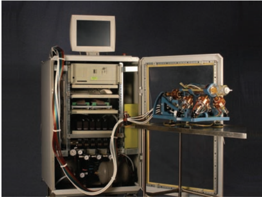
Figure 2. MrBot robot connected with 7-m-long hoses to its control cabinet.
