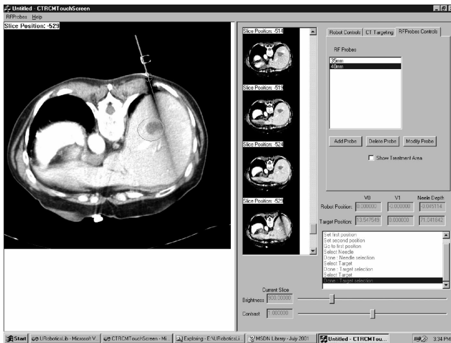
Figure 1. (a) The treatment planning system interface allows the user to select from a palette of potential ablation zones. The user indicates the position of the applicator at the skin surface and the location of the destination for the applicator tip. This information is ultimately provided to the robot for implementation. (b) Preplanning software allows testing of the expected ablation ellipsoid area against the target tumor and shows the three-dimensional nature of the expected ablation volume. In this case, a single ablation procedure would not adequately cover the entire tumor. (c) Preplanning software shows the improved tumor coverage with two overlapping ellipsoid ablation areas.
