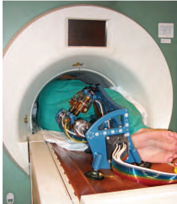
Figure 14. MR compatible robot developed for prostate brachytherapy at Johns Hopkins (simulation of a clinical procedure).
