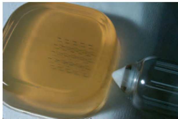
Figure 15. A 4 \times 5 \times 4 pattern of seeds with 10 mm spacing automatically placed in agar shows average seed placement errors of 0.652 mm.
