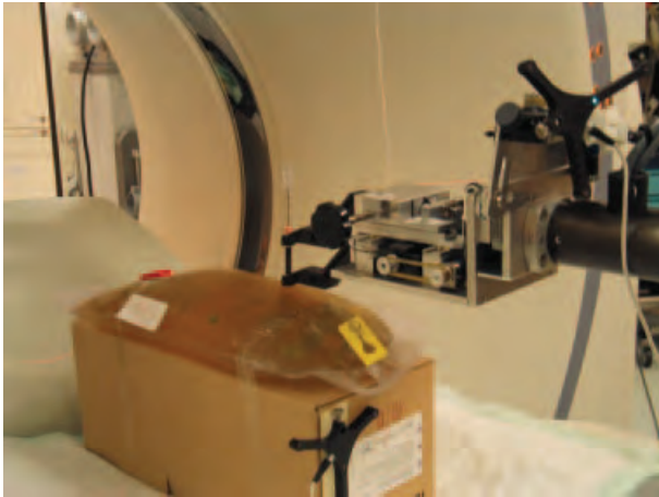
Figure 5. Close-up of testing showing phantom (peas can be seen in the bag), needle positioning unit (NPU), and optical trackers.
