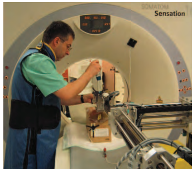
Figure 4. Biopsy robot I during in vitro testing for image-guided interventions under CT fluoroscopy.
