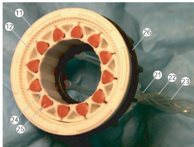
**Figure 8** Prototype harmonic motor with Tangential Wave Actuator.
