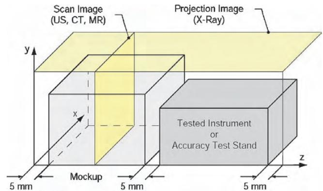
**Figure 3** Test setup for multi-imager image deterioration factor.
