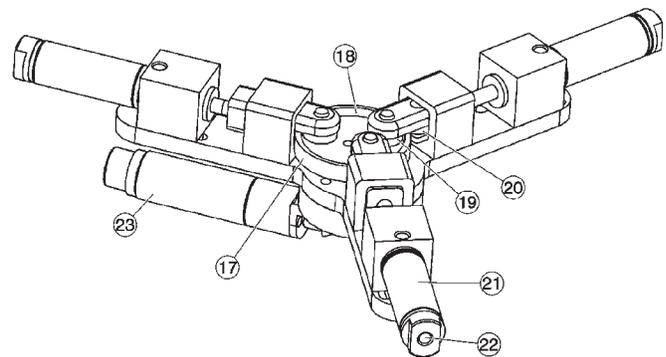
**Figure 10** Schematic of the hydraulic commutation pump.
