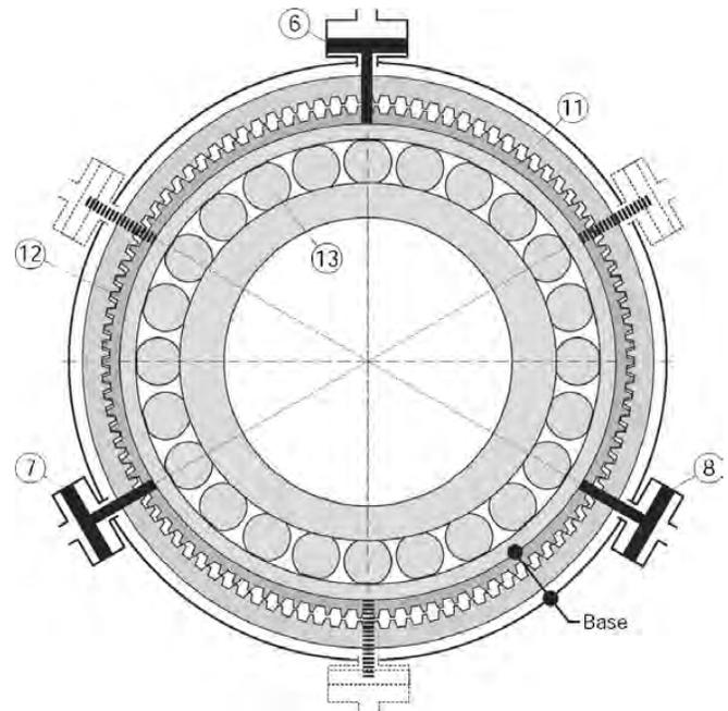
**Figure 5** Harmonic motor with rotary wave generator.
