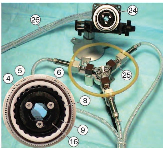
**Figure 11** Motor - pump assembly and motor detail.
