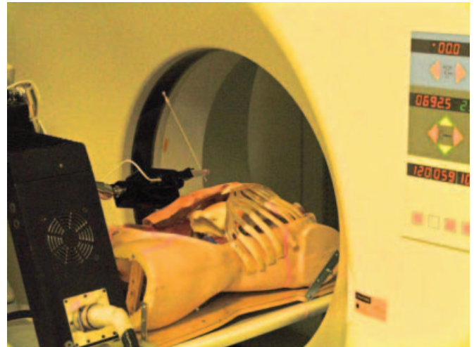
Figure 5 Robot, phantom, and needle on scan plane in CT fluoroscopy machine.
