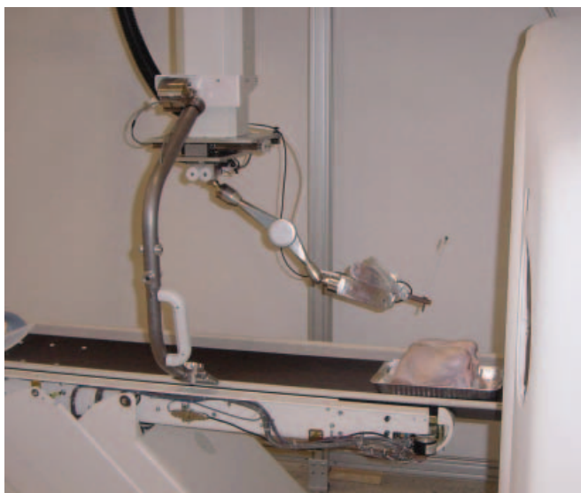
Figure 7 ImageGuide prototype undergoing testing with CT scanner.
