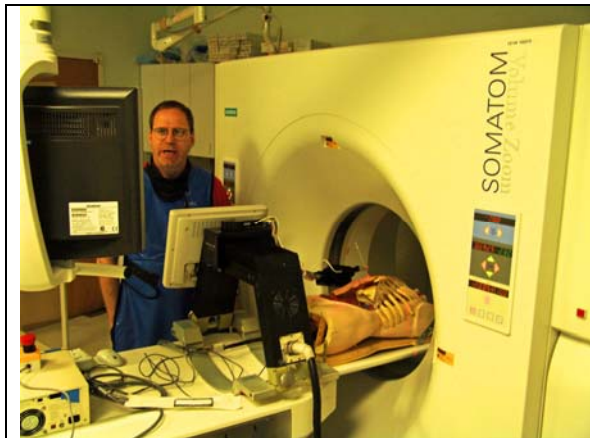
Fig. 1. Experimental setup showing CT fluoroscopy, robot, phantom, and needle on scan plane
