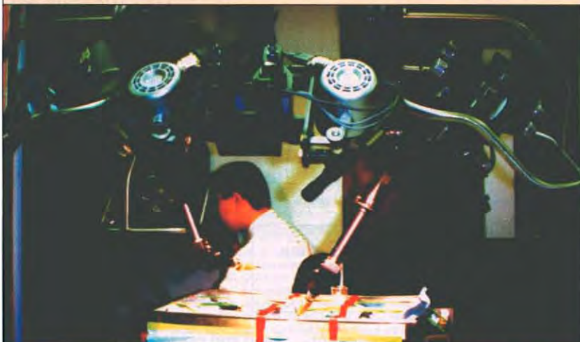
This surgeon-driven instrument manipulation system, which was designed for open surgical procedures, includes a 2-arm, high-mobility robot instrumented with grippers.
