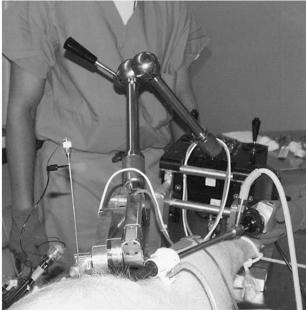
Figure 3. Impedance-needle system and robotic-positioning system during percutaneous cholecystostomy in a porcine model. Note the laparoscopic camera used to correlate needle-tip position with resistivity measurements.
