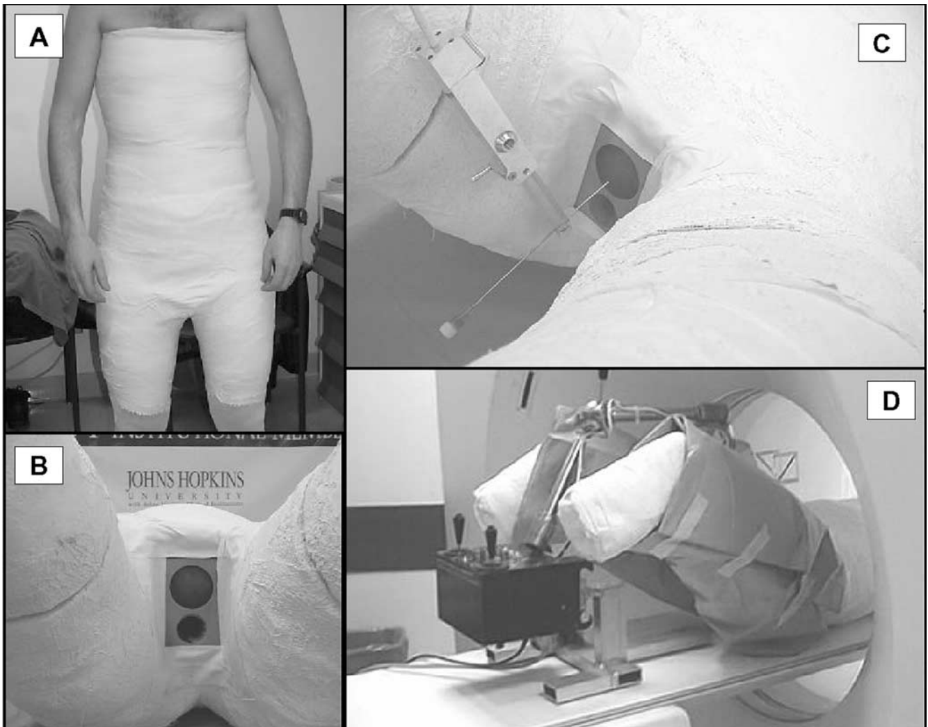
Figure 10. Anthropomorphic phantom experiment. A , Fabrication of a full-body phantom by making a plaster cast of a volunteer. B , US training phantom inserted in the pelvis of the plaster cast. C , Needle being driven robotically into the phantom through the perineum. D , Full-body phantom and robot mounted in the CT scanner.
