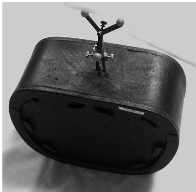
Fig. 6. Interventional phantom (CIRS, Norfolk, VA) with dynamic reference base (Traxtal Technologies, Bellaire, TX) attached.
