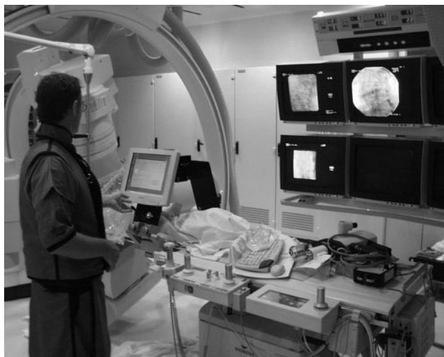
Figure 3. Physician operating joystick to control robot in cadaver study.
