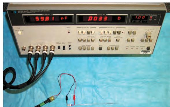
**Fig. 6.** The Smart Needle sensor of electrical impedance. [Color figure can be viewed in the online issue, which is available at [www.interscience.wiley.com](http://www.interscience.wiley.com)]
