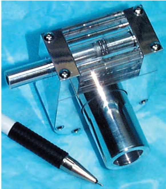
**Fig. 7.** Photograph of the prototype ball-worm transmission. [Color figure can be viewed in the online issue, which is available at [www.interscience.wiley.com](http://www.interscience.wiley.com)]
