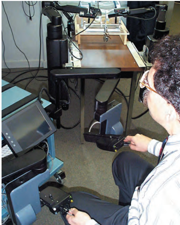
Fig. 13. Dexterity evaluation and force-feedback experiments with the Zeus teleoperation system. [Color figure can be viewed in the online issue, which is available at www.interscience.wiley.com ]
