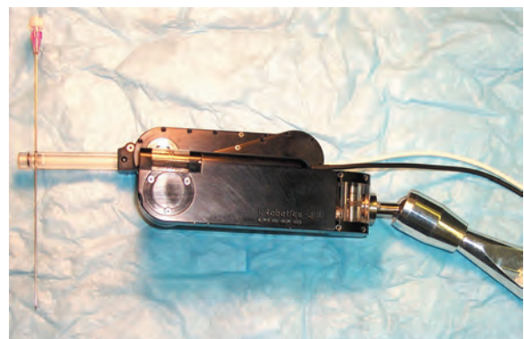
Fig. 8. BW-RCM Robot, PAKY needle driver, and supporting arm. [Color figure can be viewed in the online issue, which is available at www.interscience.wiley.com ]
