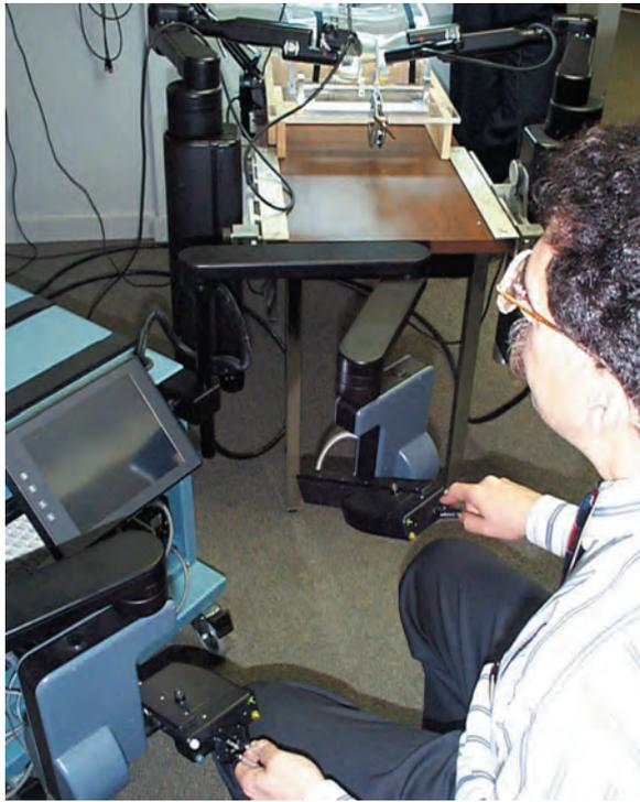
**Fig. 13.** Dexterity evaluation and force-feedback experiments with the Zeus teleoperation system. [Color figure can be viewed in the online issue, which is available at [www.interscience.wiley.com](http://www.interscience.wiley.com)]
