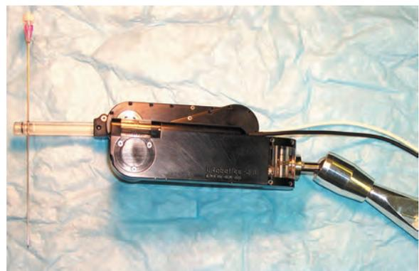
**Fig. 8.** BW-RCM Robot, PAKY needle driver, and supporting arm. [Color figure can be viewed in the online issue, which is available at [www.interscience.wiley.com](http://www.interscience.wiley.com)]
