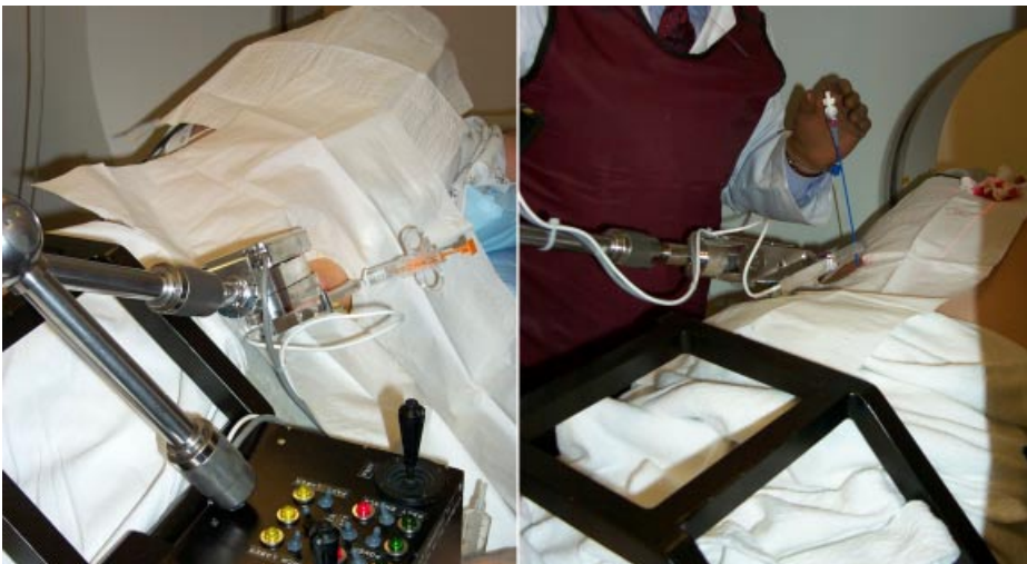
Figure 4: Robotic CT-Guided Kidney Biopsy and Nephrostomy Tube Procedures
