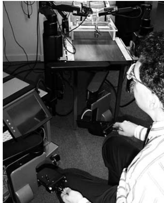
Fig. 7 Force-feedback experiments with Zeus at the Johns Hopkins Medical Institutions
